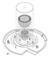
• The structure includes a roofed steel support frame that will hold aloft multiple rings of suspended metal tubes. The outer rings will form a visual veil around the structure and
